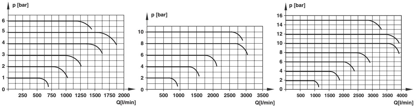
**Flow rate characteristics NG 16/connection plat ae 1/2" (NG12); P1=7 bar, 12 bar, 17 bar**
