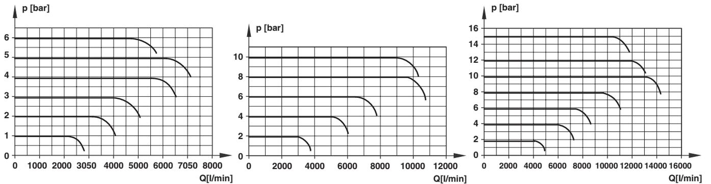
**Flow rate characteristics NG 16/connection plate 3/4" (NG20); P1=7 bar, 12 bar, 17 bar**
