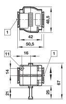
1 Main ports 1/4" or 3/8" ISO G/PTF Exhaust port M5 at 3/2 valve only
